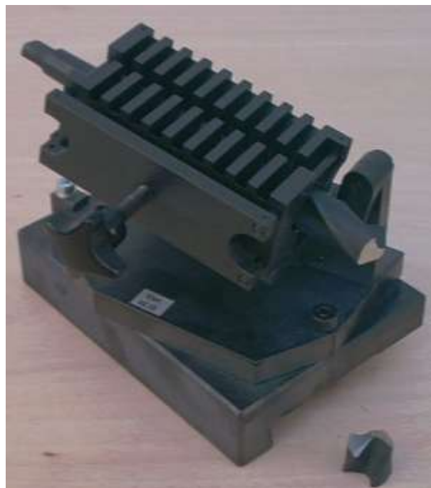
Clamping device 370.17.150.00 for cutting twist drill bits up to \varnothing 25mm. The point angle can be set from 110° to 150°.
