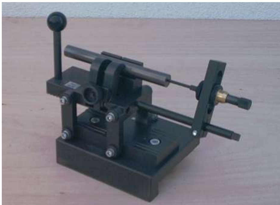
This clamping device is special as it can be swung out of the water by means of a parallelogram, without having to drain the water.
