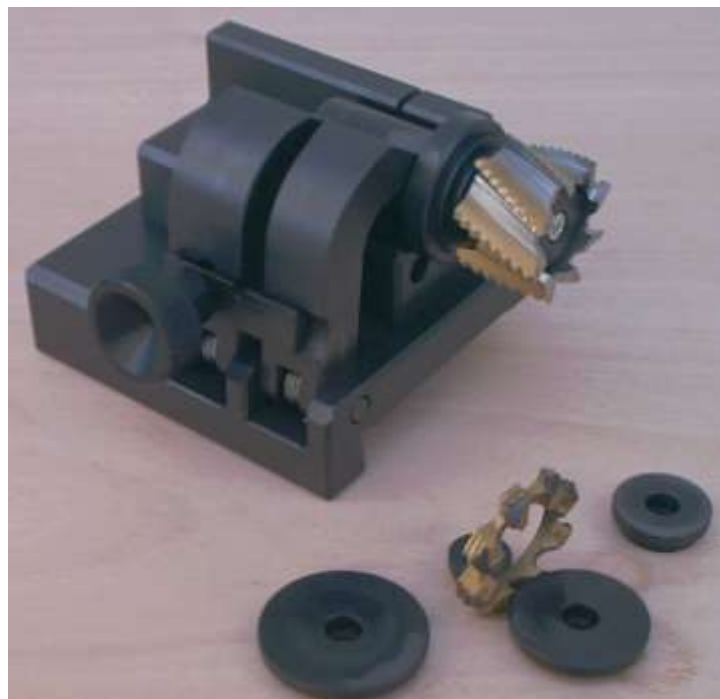
The clamping mandrel is clamped in the clamping device 370.17.100.00. Shell end mills up to \text{Ø } 125\text{mm} can be cut off in several steps by fixing the clamping mandrel by its collar on the clamping device.
