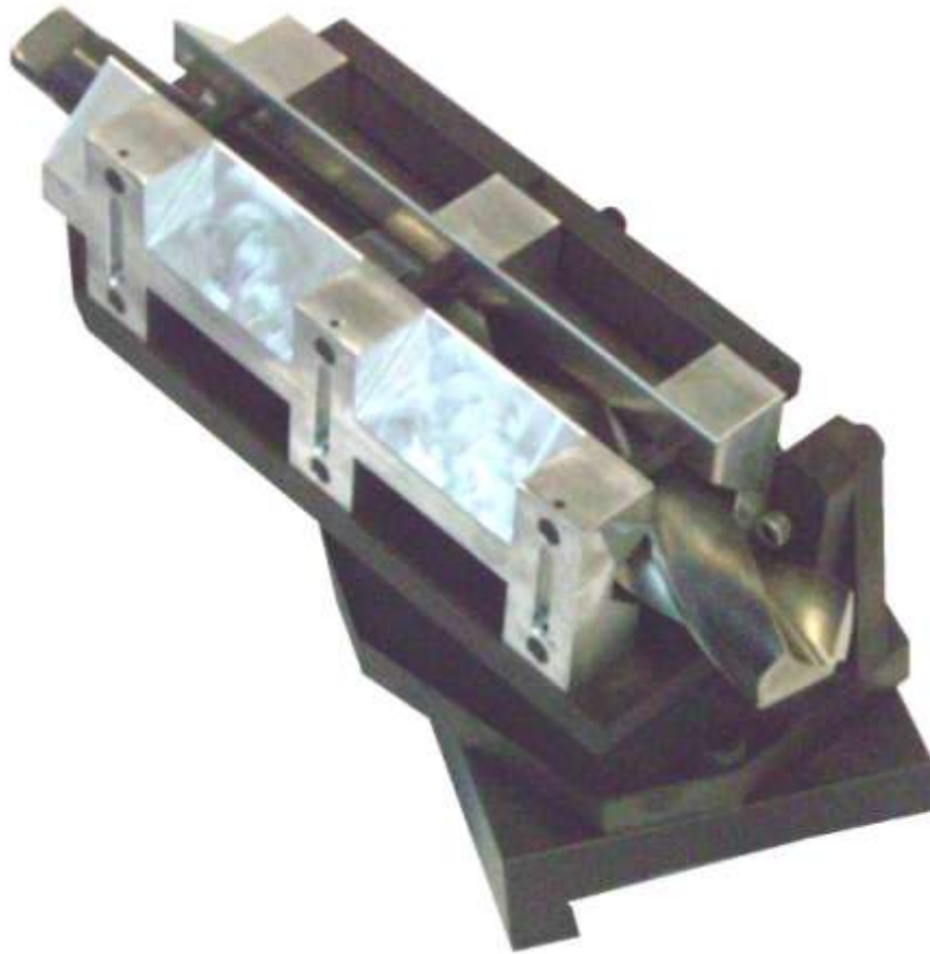
Clamping device 370.17.156.00 for cutting twist drill bits up to \varnothing 40mm. The point angle can be set from 110° to 150°.
