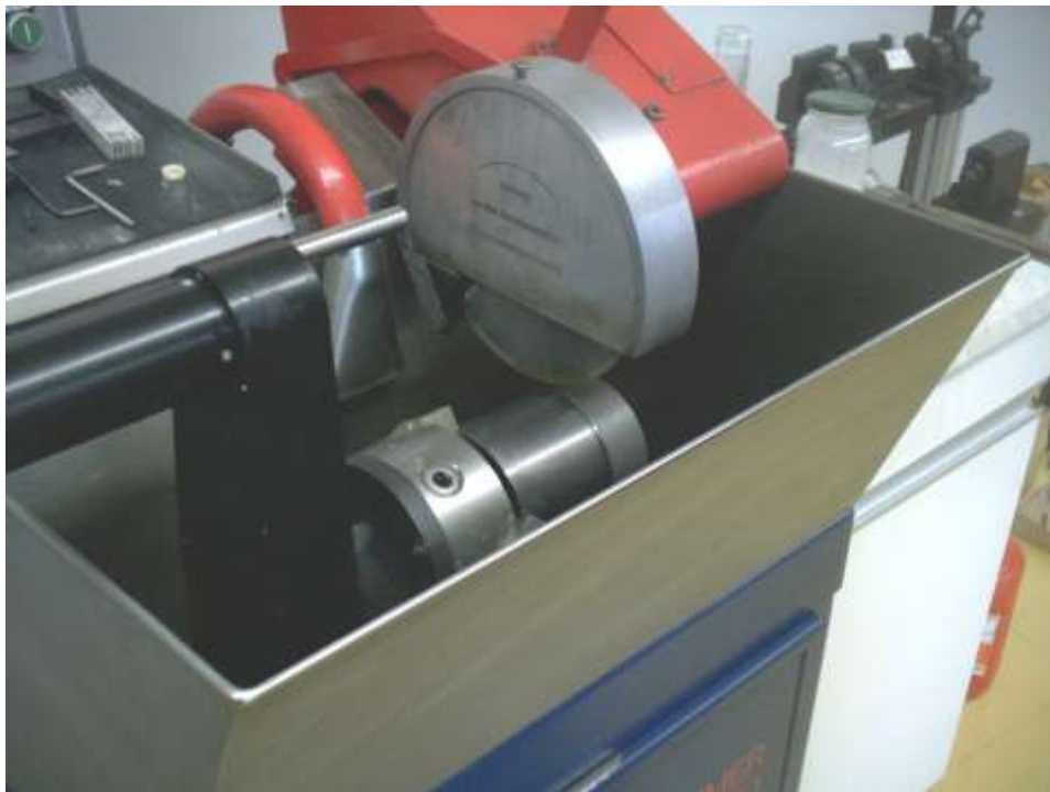
Revolving clamping device 370.17.200.00 for big workpieces up to max. \varnothing 125mm. Three-point chuck driven by electrical motor and clutch.
