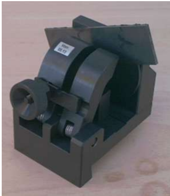
Clamping device 370.17.130.00 for 45° bevel cuts at both ends. Only for flat material at least 4mm thick.
