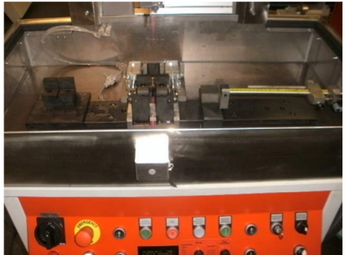
Line laser 374.90.041.00 to easily set-up various clamping devices
