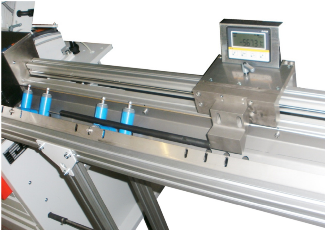
Measuring device with digital display 372.35.625.00 , here for a measuring length of 2 meters
