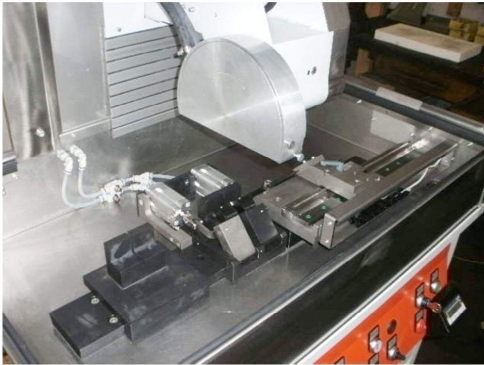
374.17.200.00 Pneumatic 3-point clamping device without carbide with built-in measuring stop with digital display 374.17.530.00
