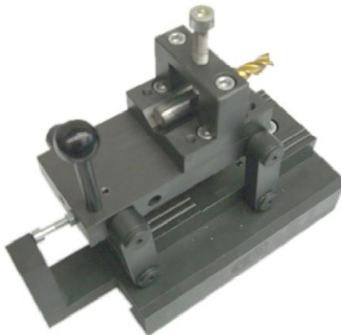
The special feature of this clamping device is that you can lift the device out of the water with a parallelogram without emptying the water
