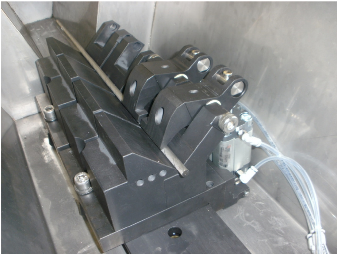
374.17.134.00 Pneumatic clamping device with V-prism
