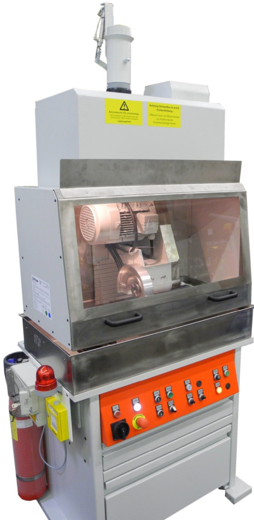
CO2 extinguisher 374.90.200.00 to work with machine oil
