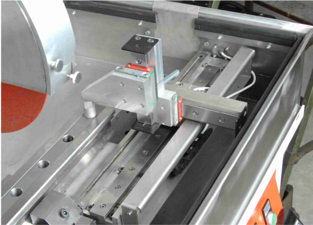
Special device 374.17.540.00 to cut-off linear guides
