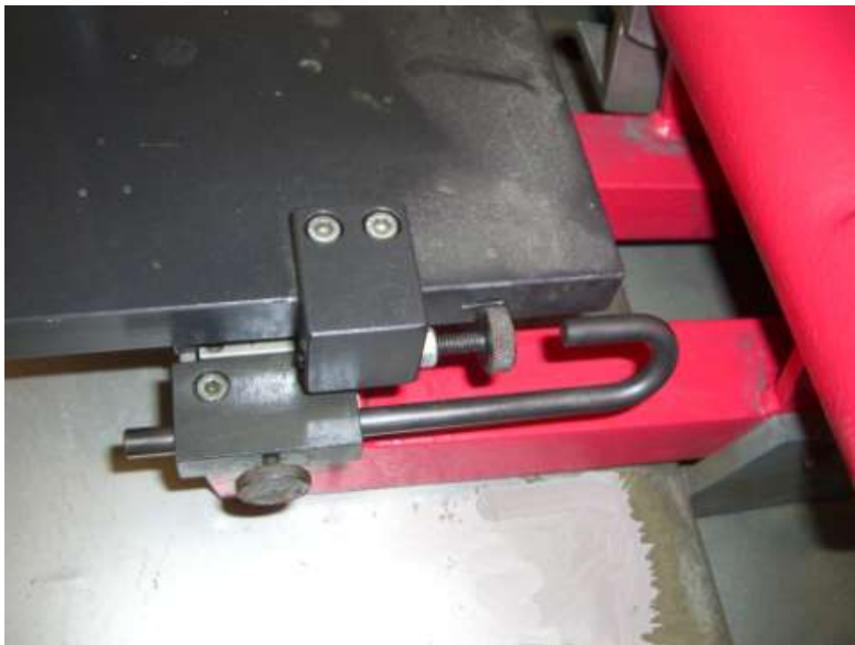
377.17.130.00 to limit the cutting depth
