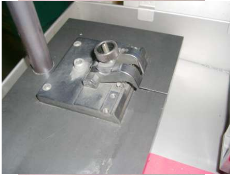
3-point clamping device 377.17.060.00 for cylindrical materials and square profiles
