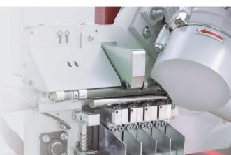
chamfers on cylindrical tools and work pieces in carbide, high speed steel, tungsten, ceramics and other hard materials. Its fast and easy operation reduces the processing costs noticeably!
